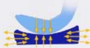
Combined stresses create subsurface fatigue
